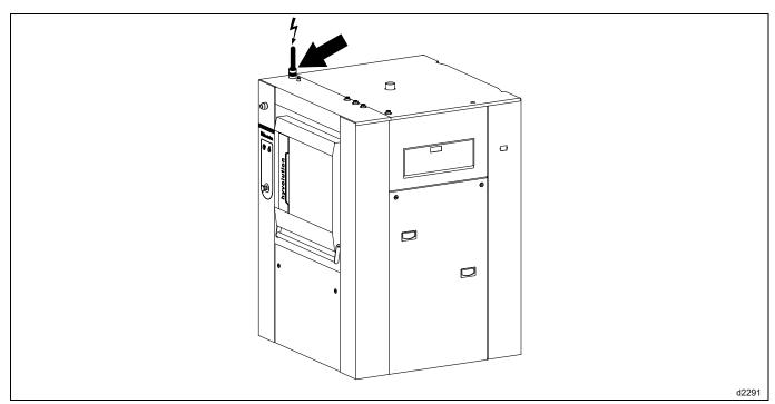
For each machine, install a fixed multipolar circuit breaker (or fuses protector) in the laundry main cabinet.
