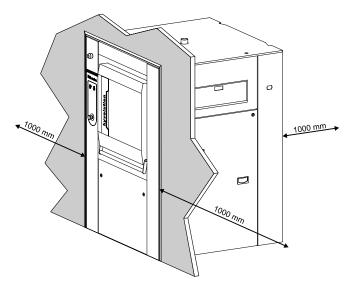
Leave at least 1 m (40") (according to the recommendation in standard EN 60204) between the machine, a wall or any other machine at the sides.
