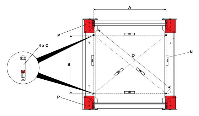
Mark out the drill holes for the securing dowels and drill them so as to insert the 4 dowels, they will secure the machine to the floor.
