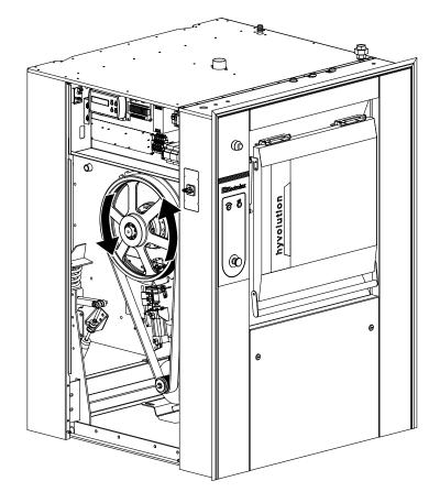
Check the direction of rotation of the circulating pump and of the draught accelerator gas heating.
